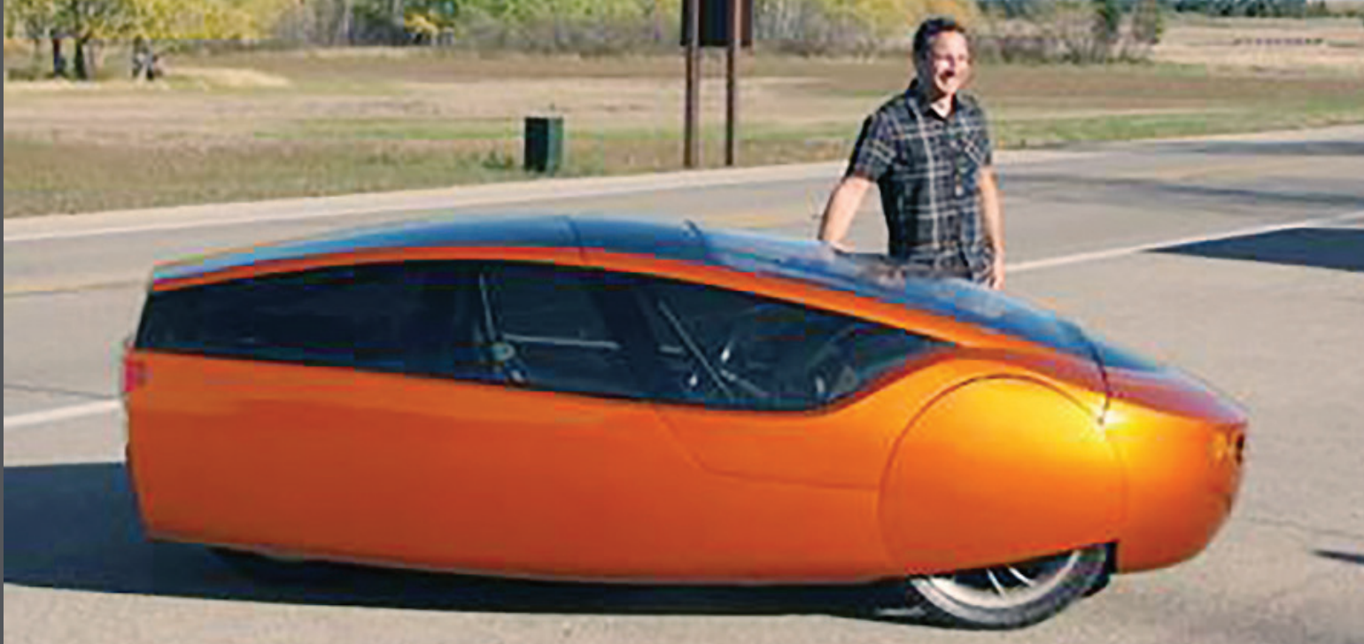
Figure 1: Full-sized car body used hot air welding and solvent to bond over 16 ABS-M30™ sections.
