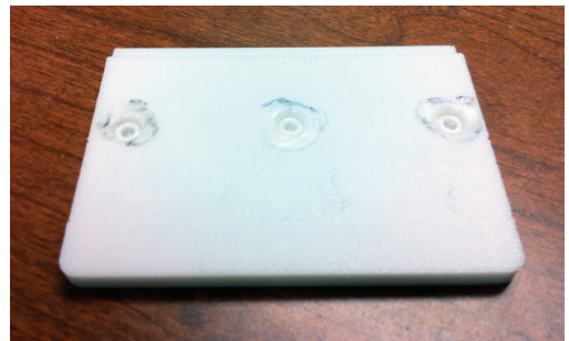
Figure 16: Spot welds from an ultrasonic welder.
