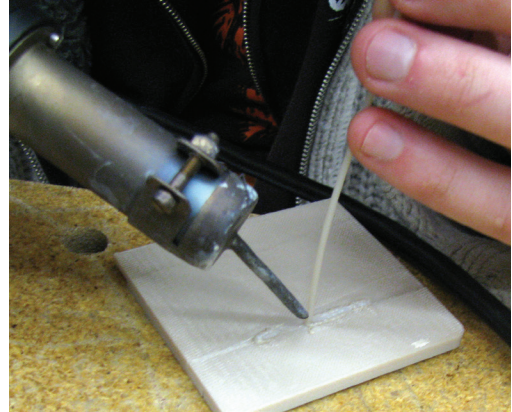
Figure 4: Draw the hot air welding tool and plastic filament along the seam.
