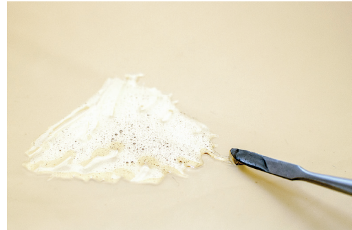
Figure 5: Mix the two components of the adhesive.
