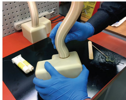
Figure 7: Mate pieces and hold or clamp.
