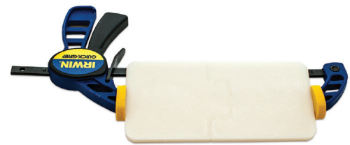
Figure 10: Align and clamp the mating pieces until the bond has set.
